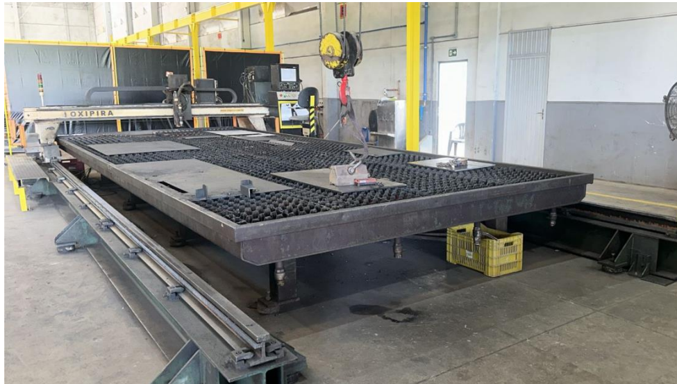
ITEM 2: APARELHO DE PLASMA OXIPIRA HYPER THERM HPR 400 XD MASTER 35
